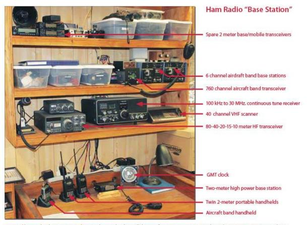
A typical ham radio "base station." There are ham radios here all the way from 80 meters (4 MHz) through 440 MHz (3/4 meters), plus a couple of aircraft radio transceivers. Everything in this picture is powered by a 12-volt aircraft battery that will hold the station up for at least 24 hours in emergency mode.
