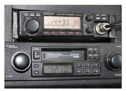
The amateur radio setup in my aircraft. The ham radio is on the top, tuned to 2-meter frequency 144.435 MHz. The radio on the bottom is an automotive AM/FM radio. Obviously, I took these pictures at 12:10 in the afternoon. Fortunately, the ham radio industry followed industry standards with 6.5-inch mounting widths.
