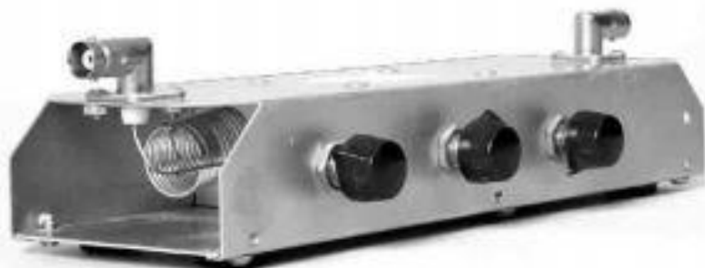
Figure 2—A view of the LGA micro relay housing.
