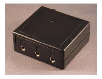
The UPK output provides a short to ground (60v max) which works nicely with any radio not having a built-in keyer, or with newer radios when connected to the key connector (set menu set to straight key, if applicable). A built-in speaker provides sound for programming the unit with a CW paddle, or listening to the programmed memory while in operation. memories are accessed with four individual memory buttons.
