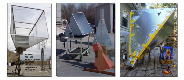
The linear polarized waveguide feeds to the horn, are relatively simple to make, but if you want to go with Circular polarization, which is in some ways better, it gets more complicated and costly. Here is a very good design and build article on a circular waveguide feed, using extruded aluminum box tubing:
