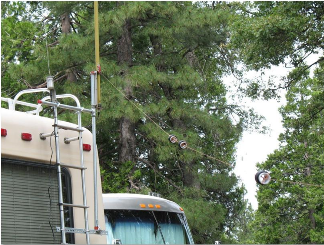
Trapped radial off the back of RV: Note the base of the 5-band vertical with homemade tilt-over mechanism that lowers the antenna to the roof
