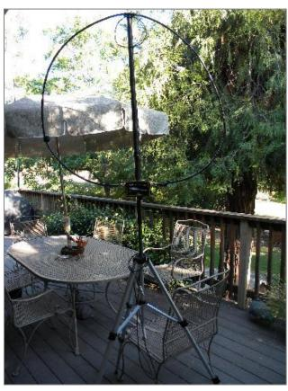
But, the noise is 2-3 or more S-units lower, and the antenna is bi-directional, and I've often been able to null the noise. Signal to noise ratio is all that counts if you can hear the signal.
