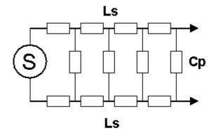
conductors separated by a dielectric. We think of an inductor as a wire wound into a coil ... the more turns, the more inductance ... but a straight wire has inductance too. Unwinding the coil until it is straight reduces the inductance, but it doesn't go to zero. Cutting the wire in half makes the inductance smaller still. But, unless the length of the wire is zero, it <u>always</u> has some inductance.
