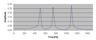
"So," I hear you say, "Those aren't exactly single frequency peaks in the plot," and you're right. I used only 1024 samples out of the number soup coming into me. Had I used more [always a power of 2], those peaks would have narrowed. Had I used an infinite number of samples, the peaks would have narrowed to infinitesimal width and it would have taken forever. None of us want to wait around until forever is over to see what our QSO buddy is typing, so we accept the approximations.
