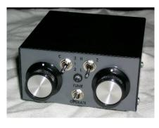
The box is 4x4x2, weighs about 9oz, and fits nicely into the nylon bag I use to carry my KX1 around. Using it is a snap. It has connectors **BNC** for input and output plus two binding posts for a balanced
