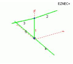
antenna for 160 or 80. We'll use it as an example. If vou remember, the Marconi-T simply a vertical radiator with a top wire that acts as capacity hat. It operates against ground
