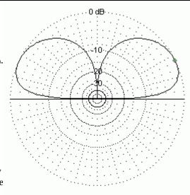
The elevation pattern is shown above. There is no gain of course, its azimuth pattern is omnidirectional, but then we don't expect short antennas to exhibit gain. The maximum radiation is at an angle of between 20 and 30 degrees which is way better than a dipole!
