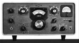
hindrance to the acceptance of SSB since doing that with a separate receiver and transmitter was more involved and difficult. And, in the KWM-2, Art Collins "went where no man had gone" in radio design. The "receiver" [i.e. what we think of when we tune a radio] covered 200 KHz from 2.955 to 3.155 MHz using an incredibly stable and linear oscillator
