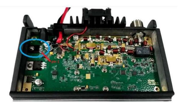
3. The LA4225 IC has five pins soldered to the board. You need to lift pin 1. I used a dental probe with a hook-end to get under the pin while I heated it with the soldering iron and it lifted right up.
