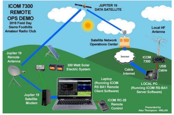
Not shown in the diagram, I had also connected a satellite-enabled ATA (analog telephone adapter) to the satellite modem to enable Remote Station VoIP telephone service. This provides an added benefit of placing and receiving conventional telephone calls over satellite in the absence of conventional phone communications.
