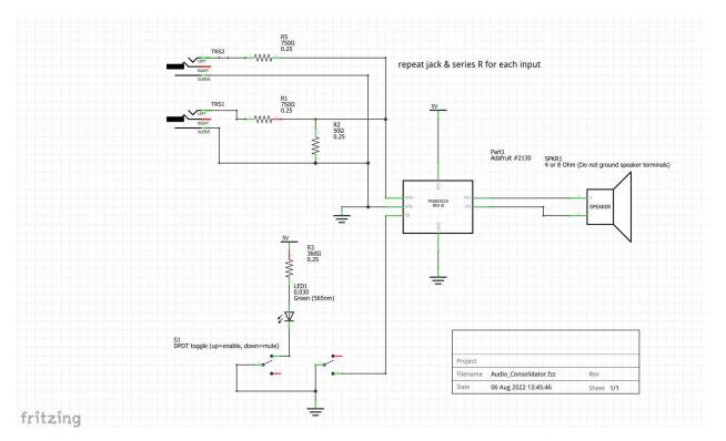
I am using 3.5mm (1/8") jacks (TRS1, TRS2) for the input/outputs. The PAM8302 has a shutdown input (SD) that I am using as a "mute" switch. I added an LED to indicate the mute status.
