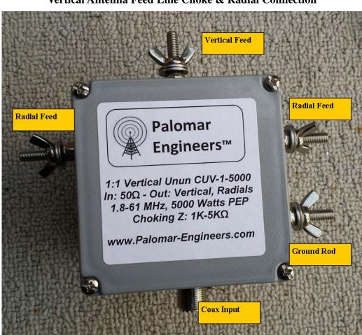
Vertical Antenna Feed Line Choke & Radial Connection
