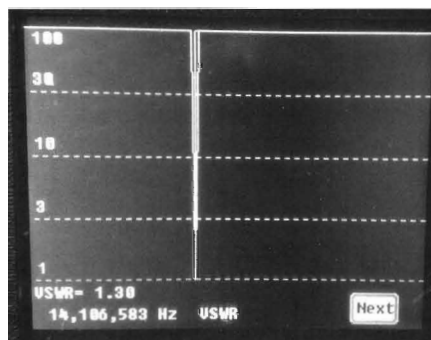
Figure 5 — Broad band VSWR Scan (10 to 20 MHz) to locate resonance.
