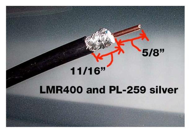
Carefully cut the black outer jacket with a dull pocket knife 1 5/16" from the end of the center conductor.
