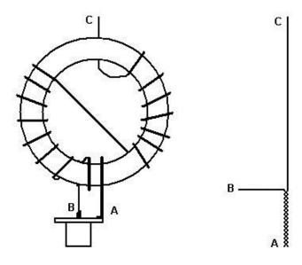
Solder a 150 pF ceramic disc capacitor, preferably 500V or better across the primary side. This cap "shortens" the antenna for 10m to compensate for the impedance of a full-wave on that band. I sourced 1kv ceramic caps from Frys Electronics that work perfectly.
