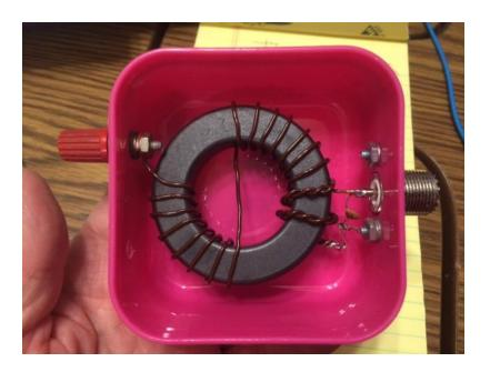
Another version built in with a water-proof electrical box (hardware store) by KM6AB showing eye-bolt strain reliefs in place.
